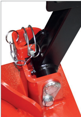
Safety pin for log-lift during transport
