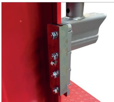
Brass slides with grease fittings
