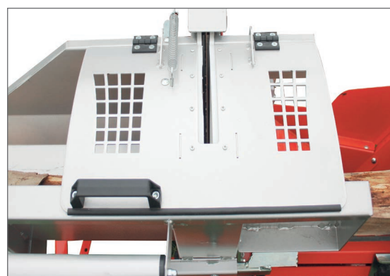
Safety cover over log carriage
