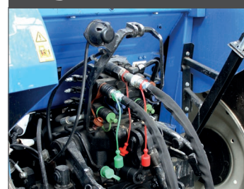
Hydraulic connection directly on the tractor
