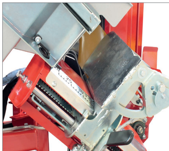
Log presence sensor for automatic sawing
