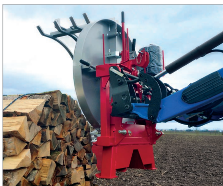
Bundler with polyester strips mechanical pivoting on 3-points hitch + euro linkage for front loader
