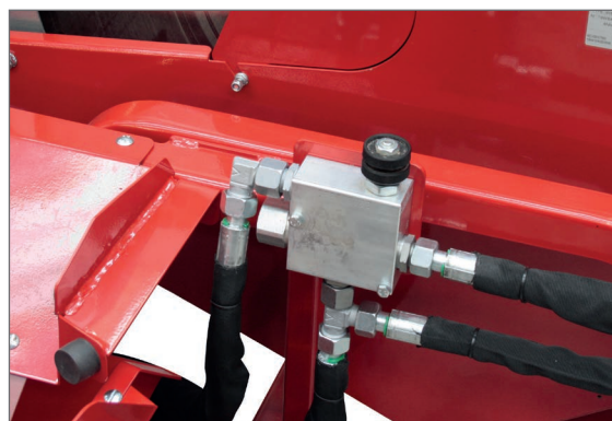
Adjustable belt discharge speed as standard on 2 SCIOMAT models
