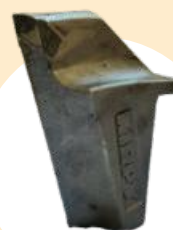
Marteau simple pastille Carbure (SP)
