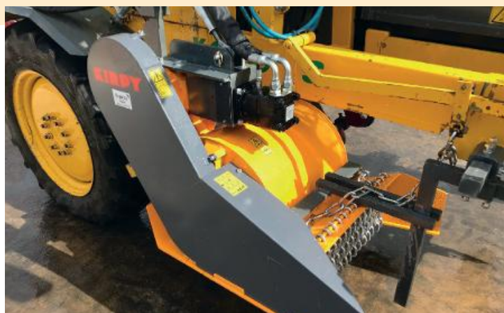
BPE 50/10 and BPE 80 designed for high-clearance tractors in either overhead or lateral position.
