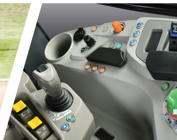
> PTO activation buttons as well as rear lift controls.
