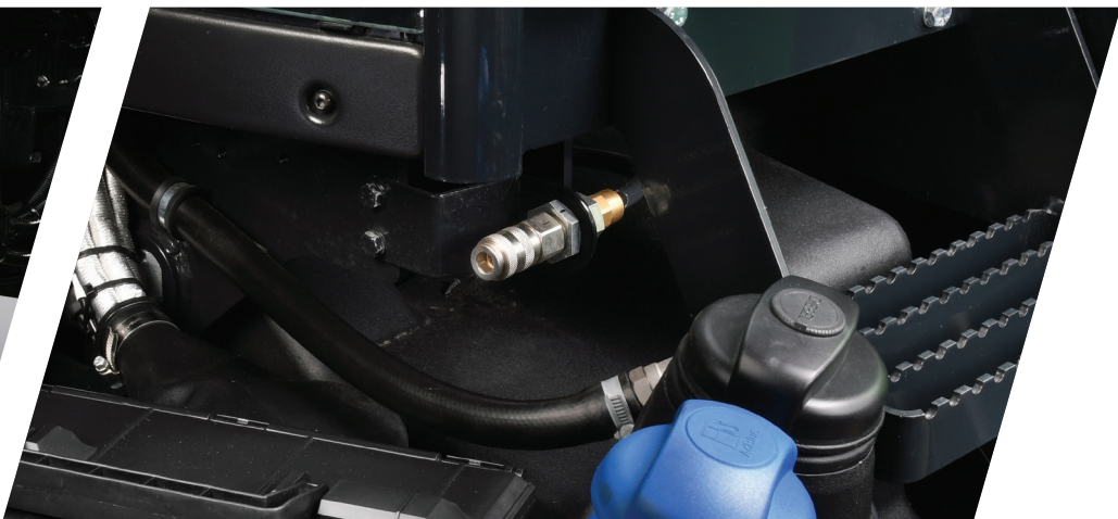
> The optional compressed air connection is located directly next to the access steps.
