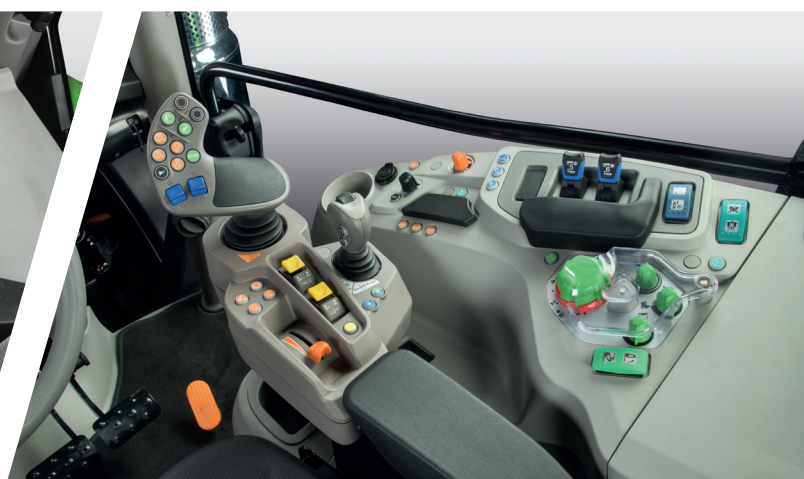
> Full electric spool valve configuration paired with TTV transmission.
