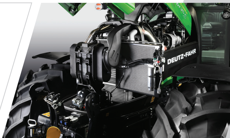
> Extendable radiator screen for easy and convenient cleaning.
