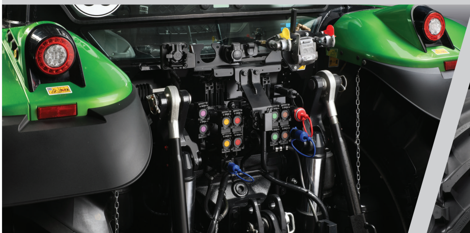
> Up to 10 rear outlets in addition to Power Beyond connectors.
