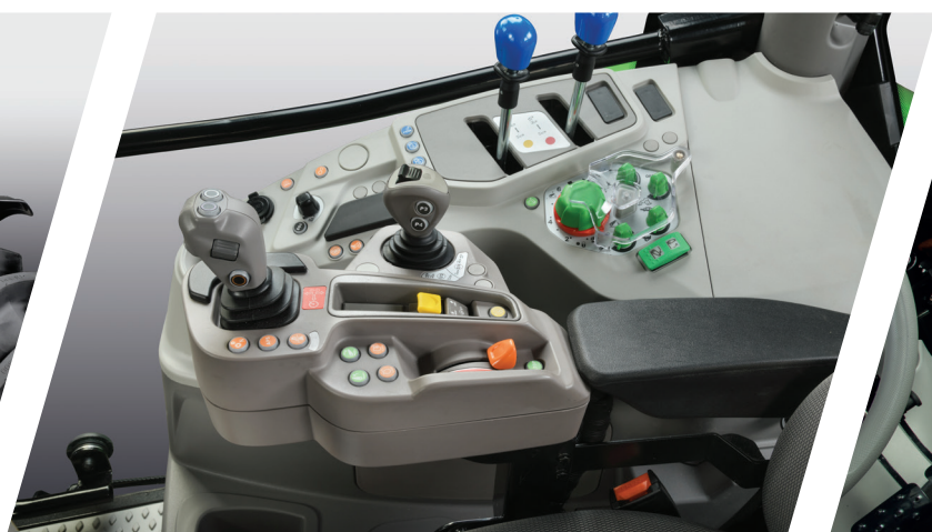
> Mixed hydraulic configuration with 2 mechanical and 2 electronic valves matched with the RVshift transmission.
