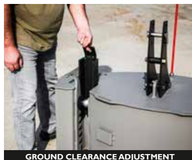
GROUND CLEARANCE ADJUSTMENT
