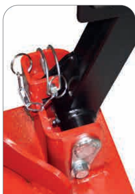
Safety pin for log-lift during transport
