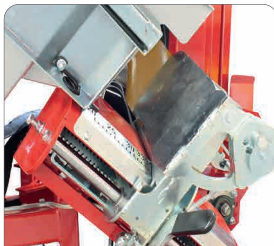
Log presence sensor for automatic sawing
