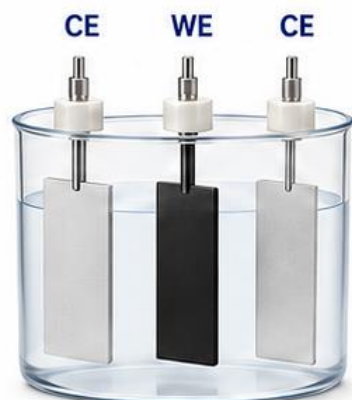
3 electrodes in a vessel WE sandwiched between 2 CE
