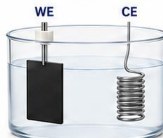
2 electrodes CE = Pt wire
