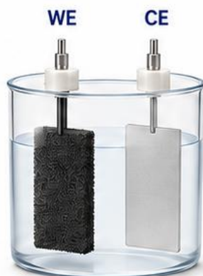
2 electrodes in a vessel High-current CE evaluation
