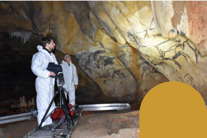
Metiscope® used by the Chauvet Cave scientific teams, enabling UV fluorescence and infrared analysis of the walls and floors.
