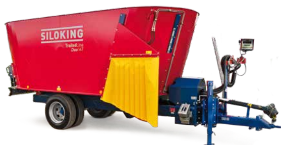
SILOKING TrailedLine Classic Duo 14-T has a total height of just 2.45 m.
