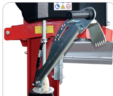
Adjustable and ergonomic wood holding claw, with gas cylinder
