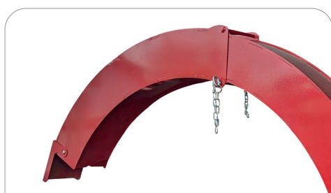
Extension of the chute to remove wood chips
