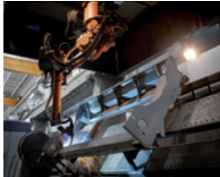
Four automated welding islands
