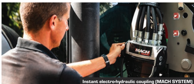
Instant electro-hydraulic coupling (MACH SYSTEM)
