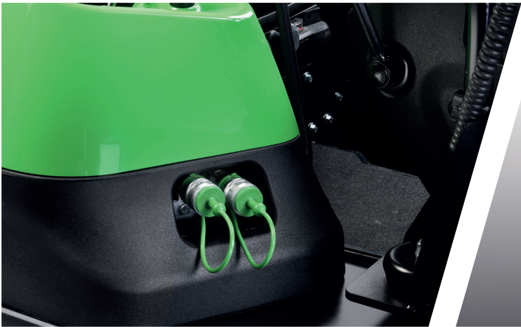
> 5 KF / 5 KM always offer 2 mid-mounted hydraulic connections.
