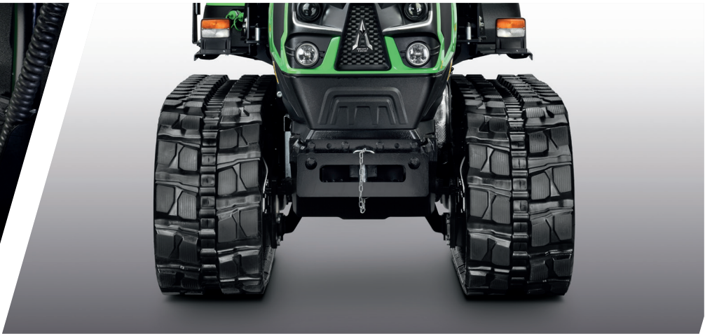
> ComfortTrack rubber tracks reduce vibrations and turf damage while keeping all the advantages of standard tracks.
