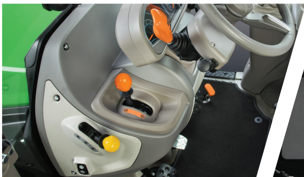
> Safe tractor parking even on hilly condition thanks to Park Lock system
