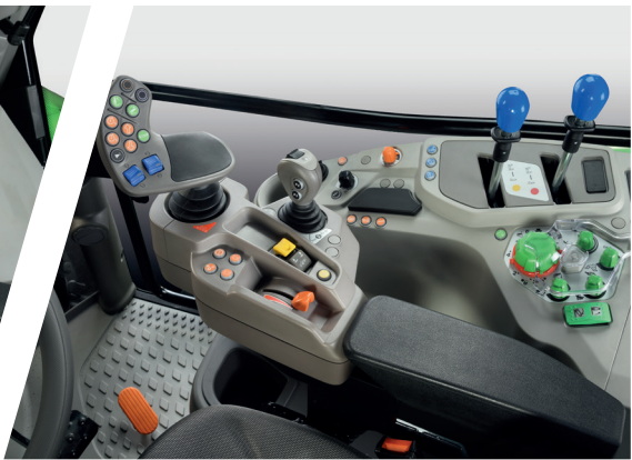
> TTV satellite armrest with MaxCom joystick.
