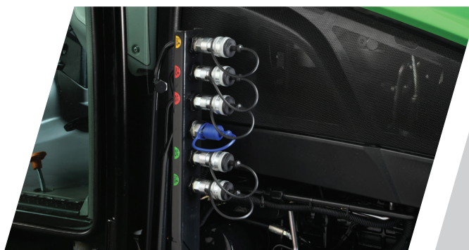
> Mid mounted hydraulic connections for front implements.
