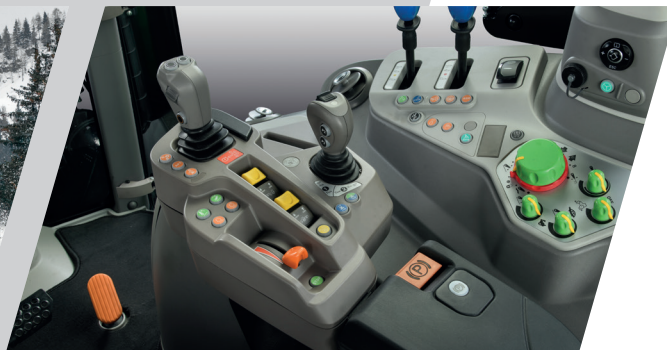
> MaxiVision* cab with RVshift transmission and mixed rear hydraulic spool valves.
