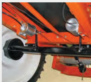
Pneumatic braking system (European homologation 167/2013)
