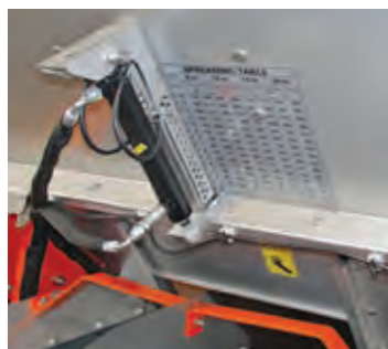
Double acting hydraulic control of fertilizer flow
