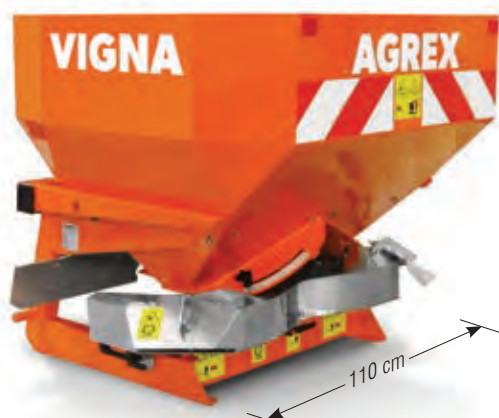
Stainless steel dual fertilizer conveyor with fast release
