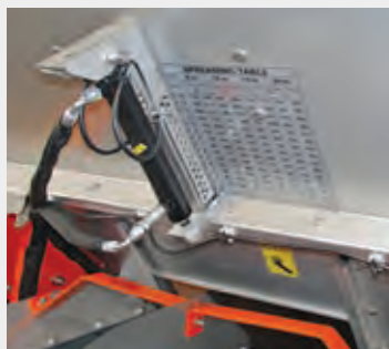
Double acting hydraulic control of fertilizer flow
