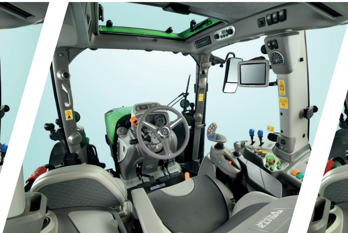
> The new MaxiVision ® cab equipment with mixed rear spool valve configuration is available for Powershift and RCshift models.
