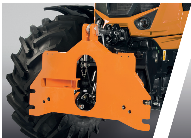
> Sauter municipal mounting (category 3/5). For fast and robust mounting of special equipment.
