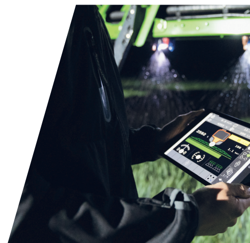
> XTEND function with tablet, control of implements via ISOBUS UT while being outside of the cabin.
