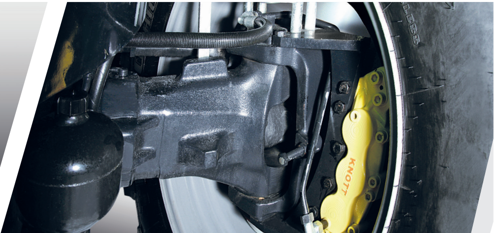
> 60 kph and maximum braking power with external dry disc brakes.
