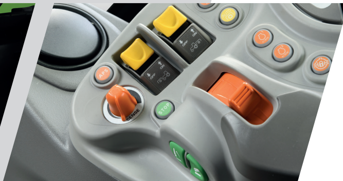
> Front and rear PTO electrohydraulically engaged and Auto PTO function.
