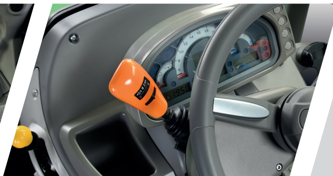
> PowerShuttle with SenseClutch.
