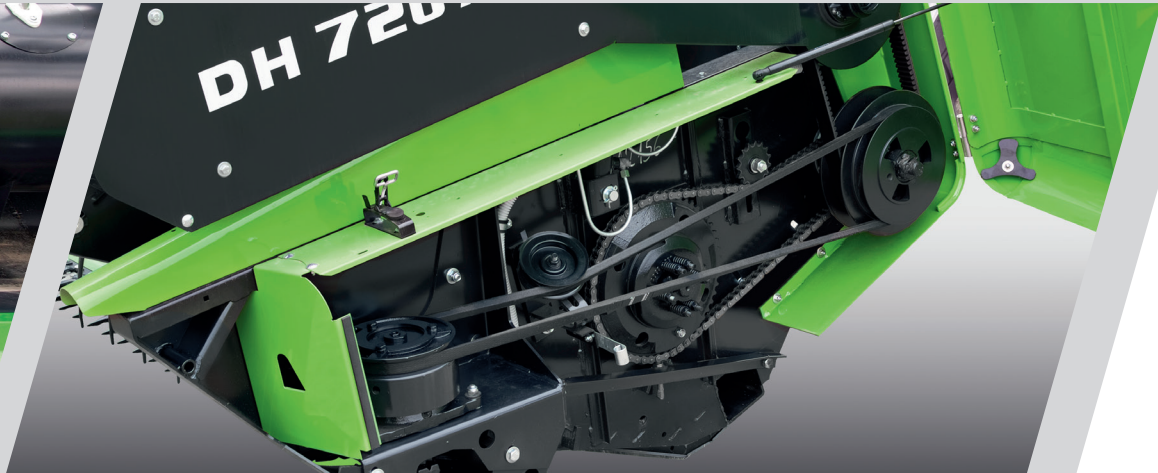
> Epicyclic gearing with 1,220 cuts/min for a high cutting frequency.
