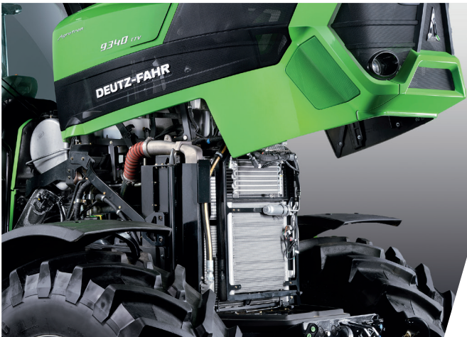
> An electrically opening hood facilitates maintenance work.
