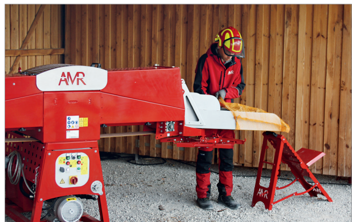
SPLITOMAT with packing table for bags of 24 or 40 L
