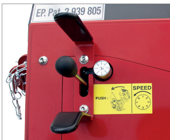
Valve and speed regulation for log carriage
