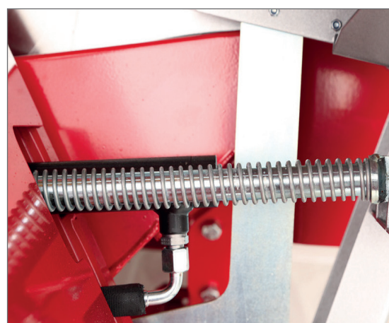
Hydraulic log carriage system
