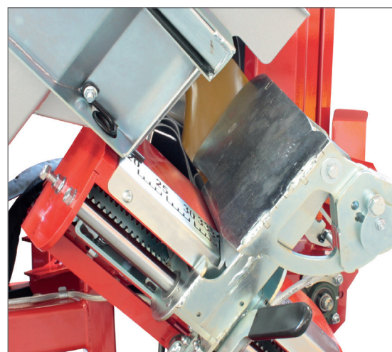
Log presence sensor for automatic sawing
