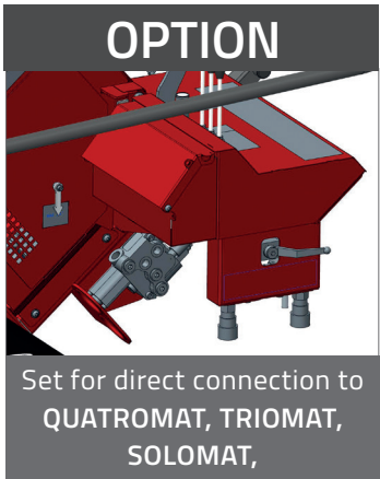
Hydraulic connection directly on the tractor
