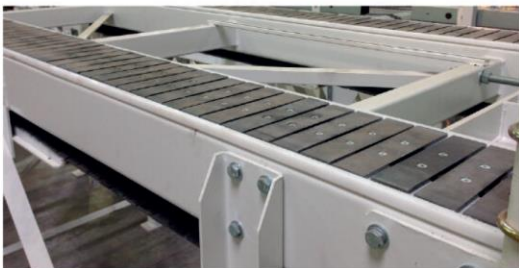
Convoyeurs tabliers Metallic frame conveyors
