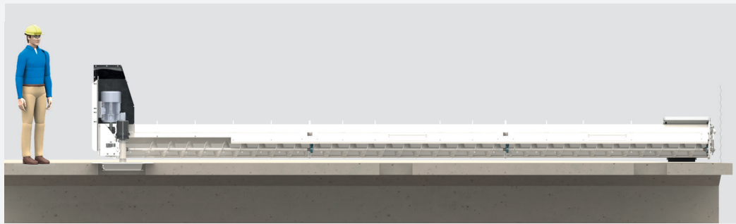
TYPE S 2 | The electric motor is inside the silo, directly coupled to a reducer driving the auger. Power is supplied by a rotary collector.
