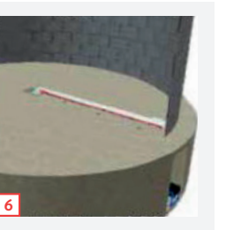
Step 2: Starting and 360 degrees rotation of the sweep auger
