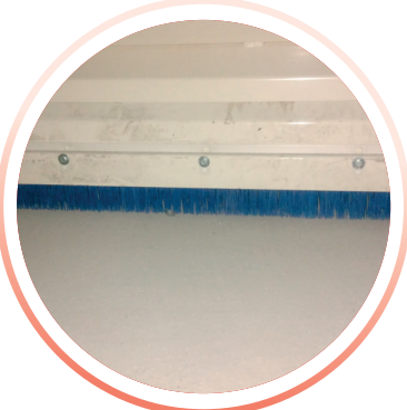
CLEANING BRUSHES Combined with a good quality concrete floor, reduce the remaining layer of product to an insignificant quantity.
