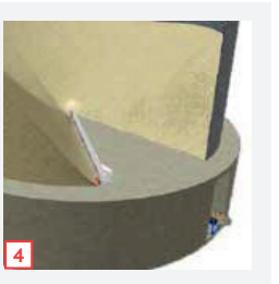
Step 2: Starting and 360 degrees rotation of the sweep auger
