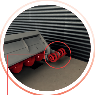
CLEARING SCREW To clear the Advance Wheel path of product wastes on the silo periphery (included for large silo diameters and dusty products).
