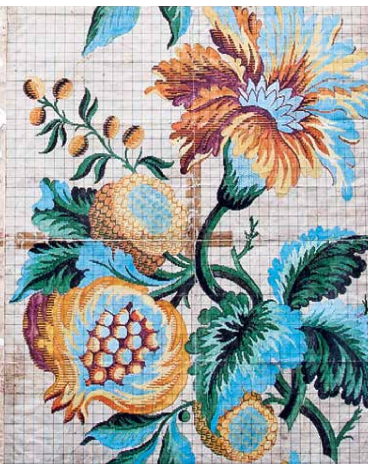
^ Messa in carta per telaio jacquard. Weave draft for Jacquard looms.
